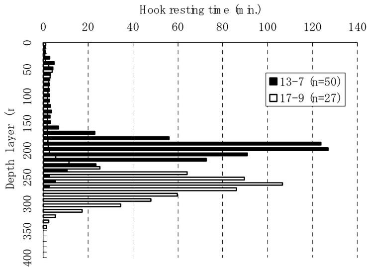
Fig. 2 Estimated distribution of hook resting time by 10 m depth layer of 7th line in Number of hooks between float (NHF) =13 (13-7) and 9th line for NHF=17 (17-9). Calculated depth of hook by catenary model was 200 m for 13-7 and 240 m for 17-9 respectively. 'n' means the number of TDR data available from one operation.
