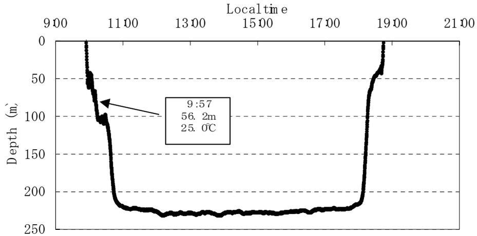
Fig. 1 Example of time-depth data of longline hook when Atlantic blue marlin was caught by a next deeper branch line with probe. Data collected in 4th of November 2000 in position in 4.6 S and 17.6 W.
